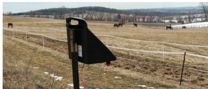
Many solar chargers have a handy ready-made slot for mounting on a T-post.
